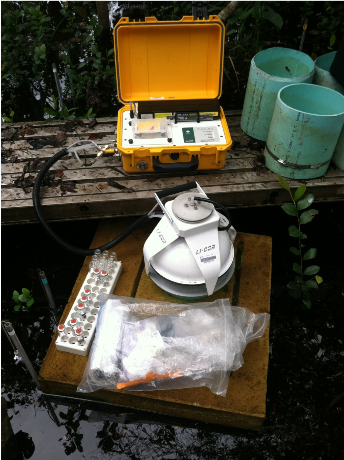
Figure 9. Photo of LICOR LI-8100 IRGA sampling above flooded soils, with installed pore-water sipper tubes also featured to the left of the floating platform and IRGA.
