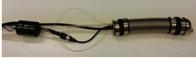
Figure 5: ARC Peristaltic Crawler
