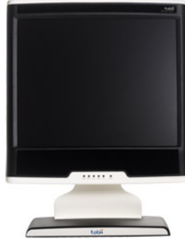
Figure 5.3: Tobii T60 eye-tracking system that was used to monitor the real-time pupil sizes of the subjects during the tests.
