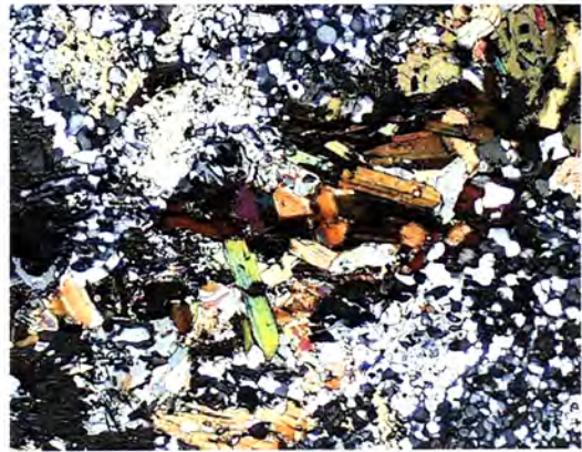
Figure 41: Photomicrographs of phlogopite. Photomicrographs in plane and cross polarized light of phlogopite crystals in gabbroic xenolith sample 12-20-3. Field of view 2.8 mm.
