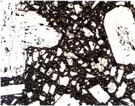
Figure 19: Photomicrographs of andesite. Photomicrographs in plane and cross polarized light of andesite. Field of view is 2.8 mm.
