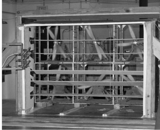
Figure 3.2 Six-fan WoW Small-scale (1:8) model.
