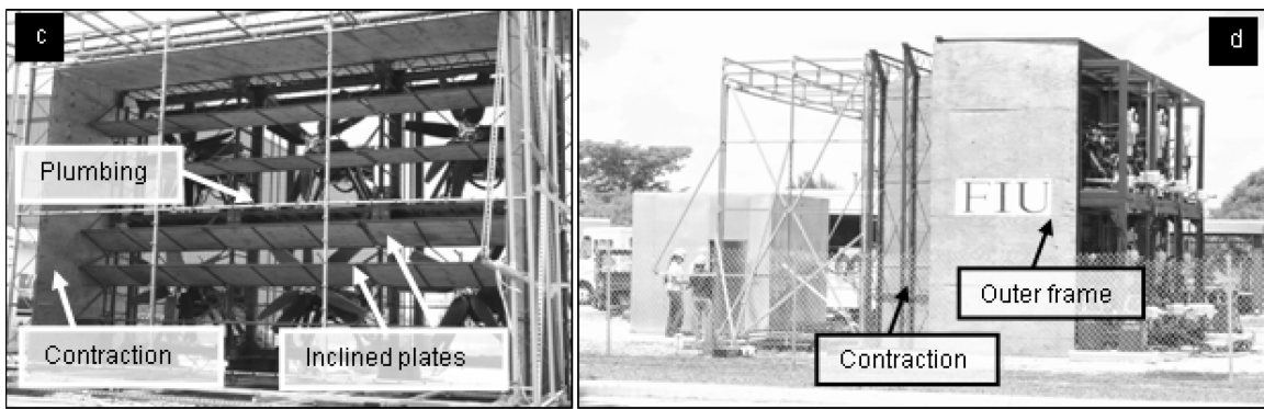
Six-fan Wall of Wind: (c) front view and (d) side view
