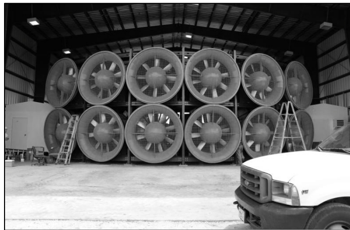
(f) The new twelve-fan Wall of Wind
