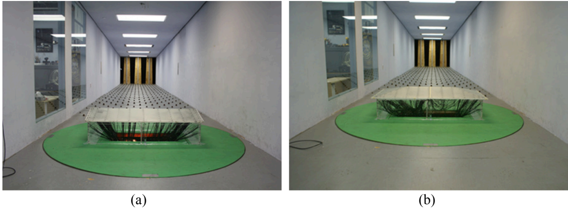
Figure 4.2 Wind tunnel testing set up for low-rise building with (a) Gable and (b) Hip roof.
