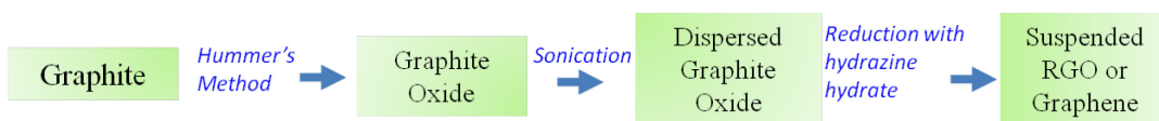
Figure 2.5: A schematic representation of the process steps of graphene synthesis by chemical method [Reprinted with permission from Reference 46 ].
