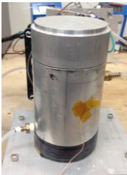
Figure 4-3 The structure of the small self-fabricated hydrogen furnace
