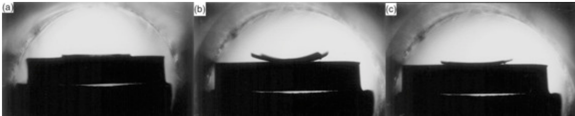
Figure 3-8 Photos of camber development for the Ag/LTCC (A) room temperature, (B) 750 °C, (C) 850 °C [136]
