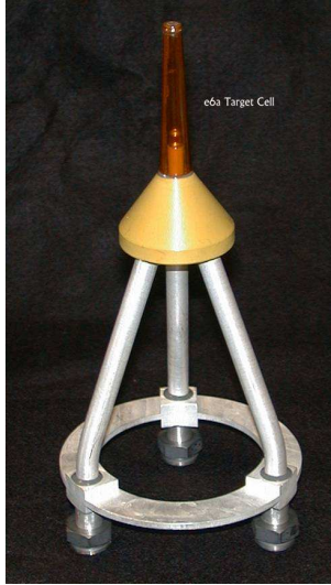
Figure 2.9: E1F cryogenic target.
