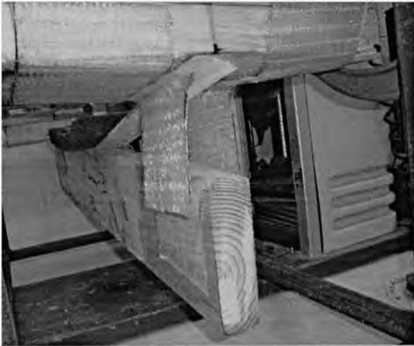
Figure 3.28 – Failure of specimen strengthened with straps
