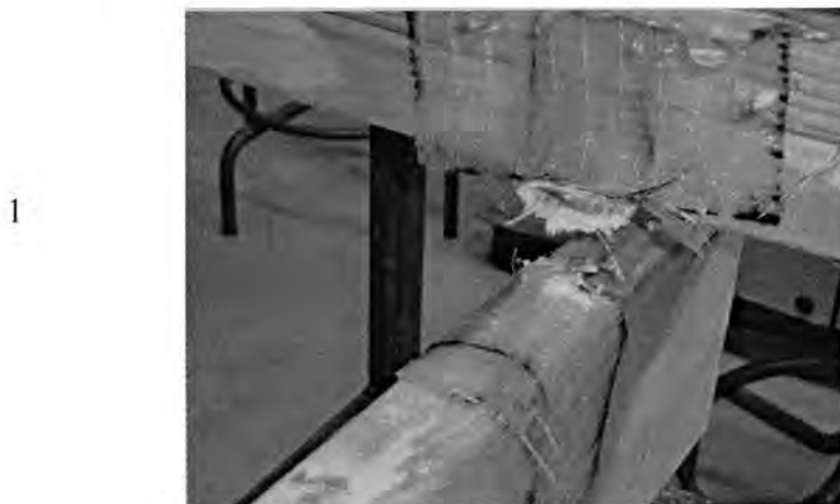
Figure 3.11 – Failure of FRP tie Configuration II
