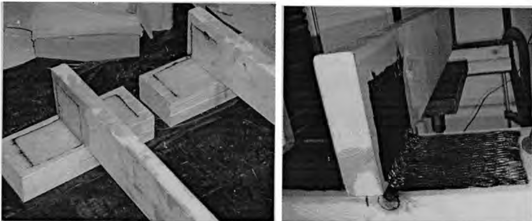
Figure 3.18 – Configuration A with GFRP (left) and CFRP (right) before testing
