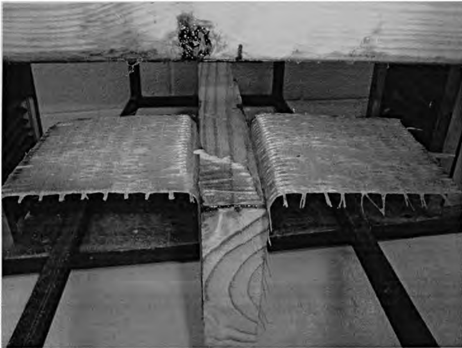
Figure 3.31 – Failure of specimen with SYP wood
