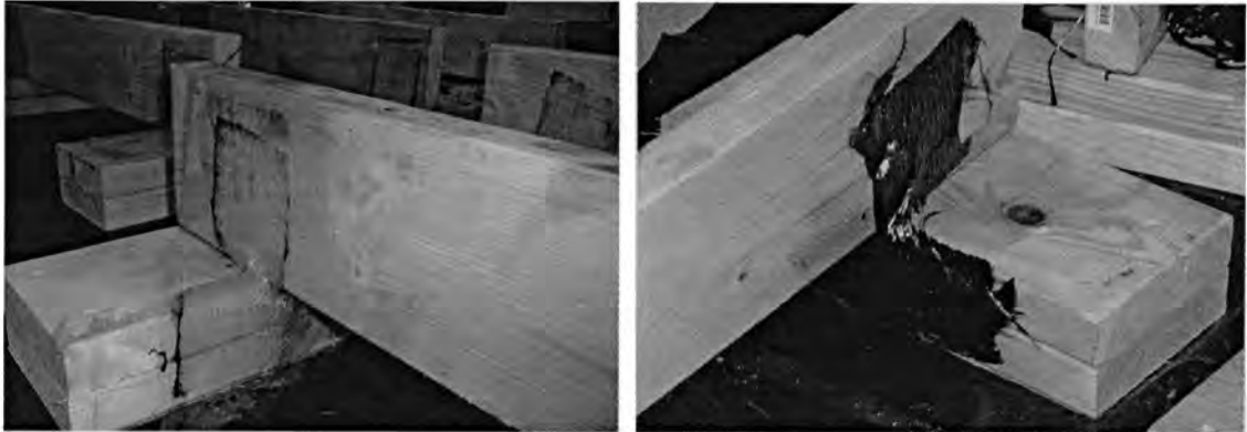
Figure 3.20 – Configuration B with GFRP (left) and CFRP (right) before testing
