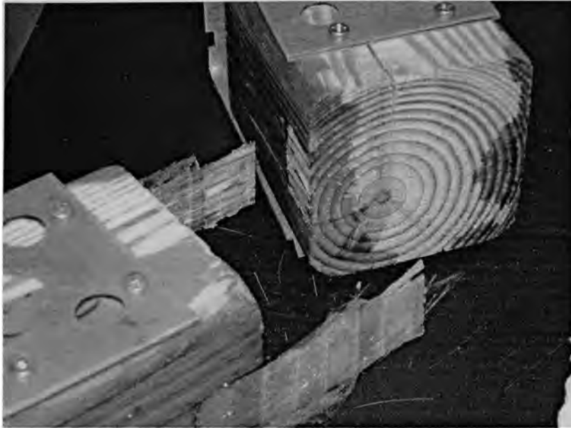
Figure 3.3 – Typical failure of direct shear specimen
