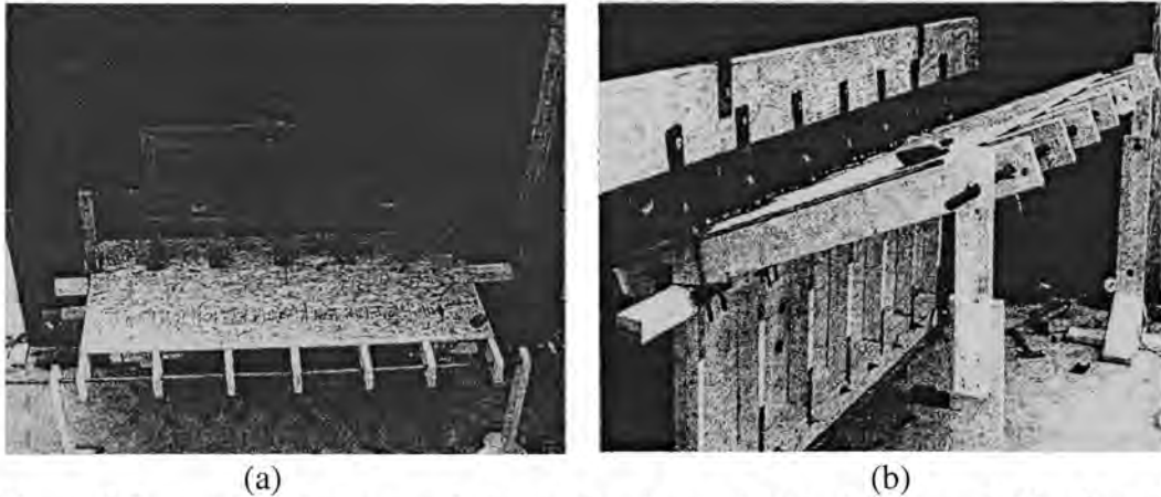
Figure 2.9 – (a) Specimen consisting of 7 rafters, (b) Load tree used (Reed et al.
