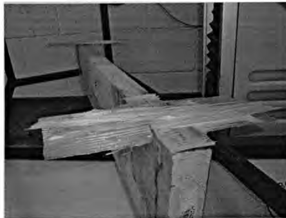
Figure 3.17 – Failure of FRP tie Configuration V
