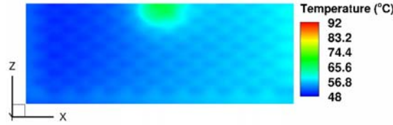
Figure 42. Temperature distribution on the top surface of the top wall of the array of micro-pin fin array having airfoil cross section pin fins with: a) 5\ \mu\text{m} , b) 10\ \mu\text{m} and c) 15\ \mu\text{m} graphene nano-platelets heat spreader.
