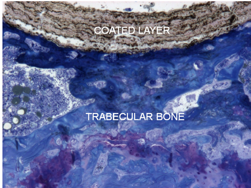
Figure 4.51: Histological image (5X) of HA-CNT coated implant in rat, with toluidine blue coloration, shows HA-CNT coating strongly attached to newly grown bone tissues.
