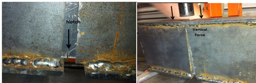
Figure 4.1 Process of crack formation
