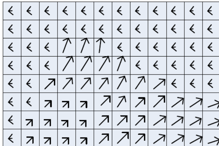
Figure III-13 Typical Motion Vector MB map in H.264 encoding
