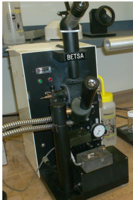
Figure 3. 3: Drilling machine which is employed to drill holes in the gaskets using spark erosion method.
