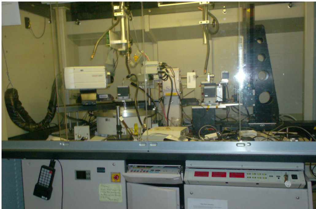
Figure 3. 6: A Bruker- GADDS/D8 X-ray system with molybdenum rotating anode X-ray generator at CeSMEC.
