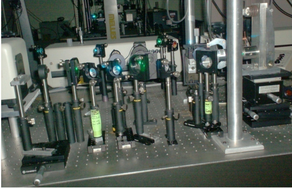
Figure 3. 7: Raman spectroscopy setup with in situ ruby pressure measurement system at CeSMEC.
