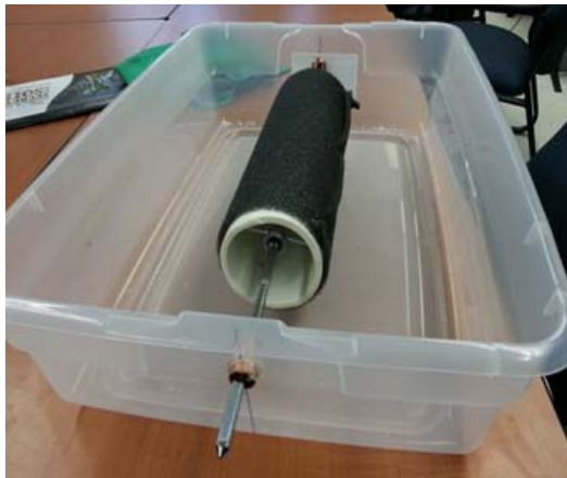
Figure 8. Semi-Submerged, Rotary System
