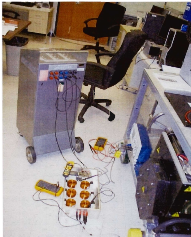
Figure 4.1-3 Experimental setup for AVR and frequency response verification of the alternator
