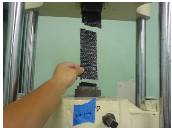
Figure 5.6 Failure Mode of CH-I-4: LWV
