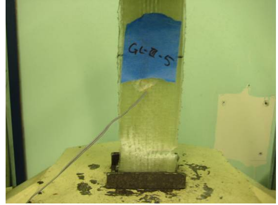
Figure 5.46 Failure Mode of GL-III-5': LAB
