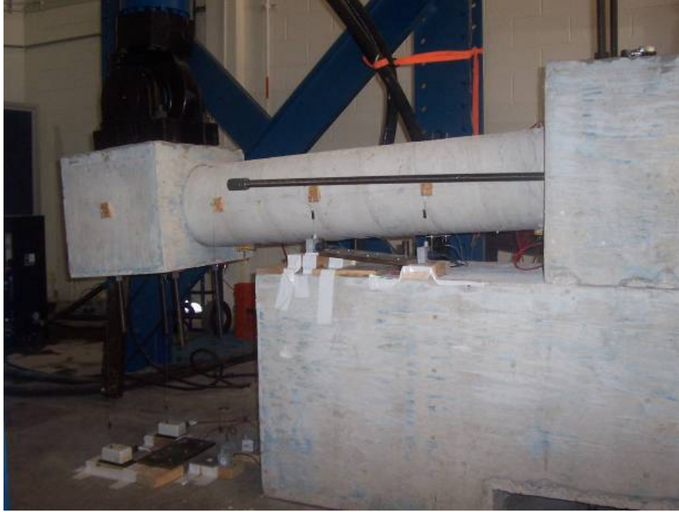
Figure 3.42 Specimen RC at \mu of 10 without Axial Load
