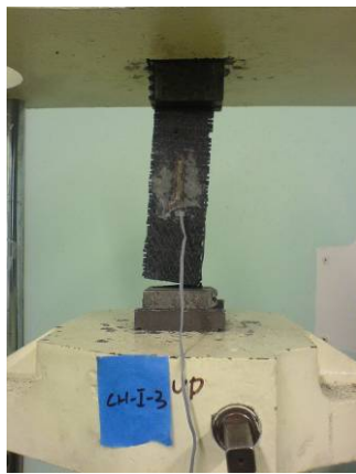
Figure 5.5 Failure Mode of CH-I-3: LWV
