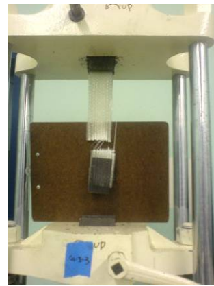
Figure 5.38 Failure Mode of GL-I-3': LAB
