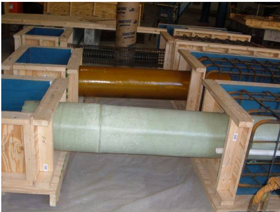
Figure 3.8 Overall Embedment into the Column Heads and Footings of Specimens G, Y and RC
