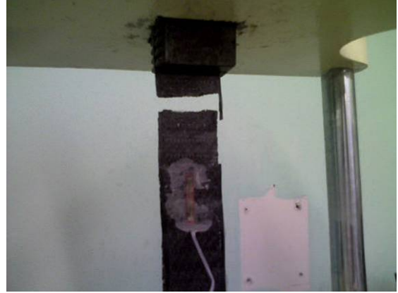
Figure 5.10 Failure Mode of CH-II-4: LVV
