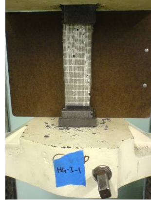
Figure 5.52 Failure Mode of HG-I-1: SGM
