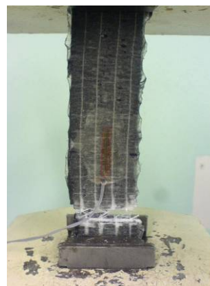
Figure 5.62 Failure Mode of HL-V-2: LWB
