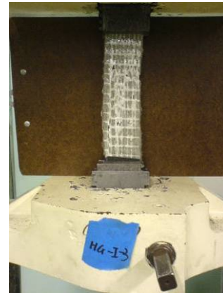
Figure 5.54 Failure Mode of HG-I-3: SGM
