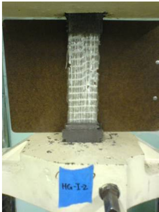
Figure 5.53 Failure Mode of HG-I-2: SGM
