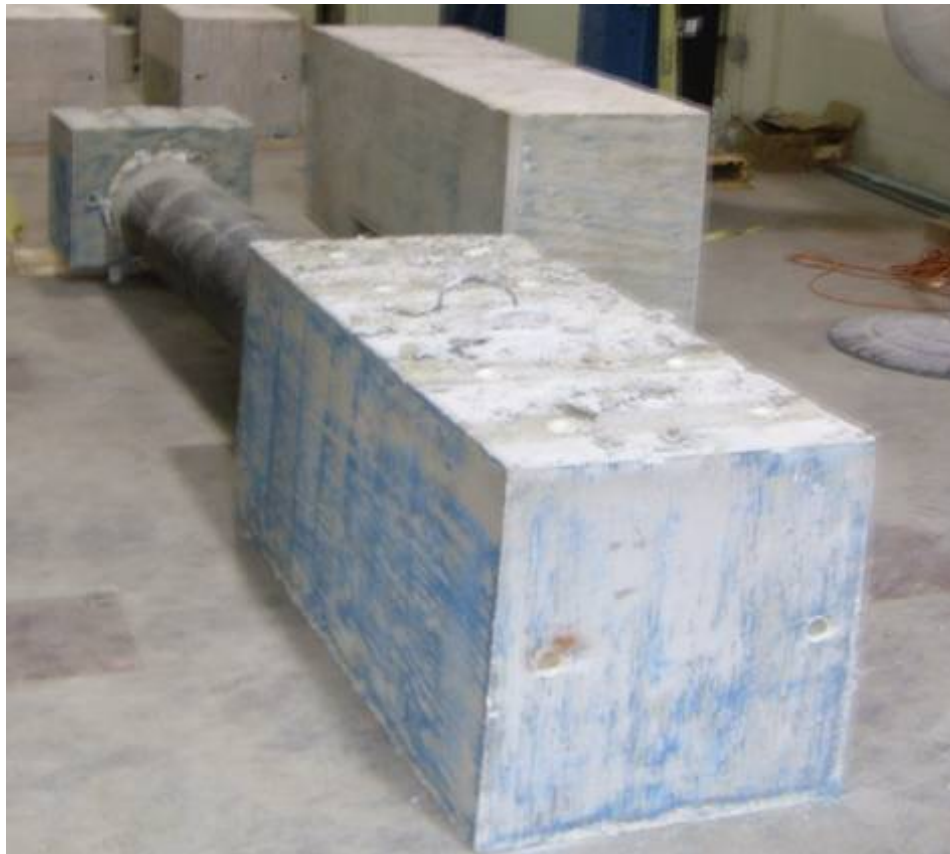
Figure 3.14 Specimen LC and Pedestal after De-Molding
