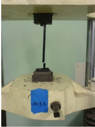
Figure 5.51 Failure Mode of HC-I-5: SGM
