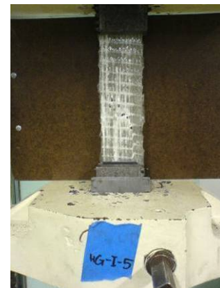
Figure 5.56 Failure Mode of HG-I-5: SGM
