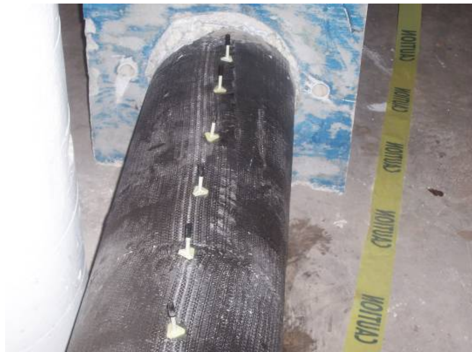
Figure 3.19 Specimen after Epoxy Injection
