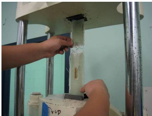
Figure 5.43 Failure Mode of GL-III-3: LIT
