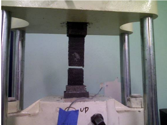
Figure 5.3 Failure Mode of CH-I-1: LGM
