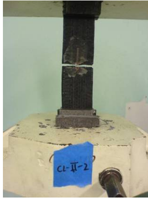
Figure 5.21 Failure Mode of CL-II-2: LGM
