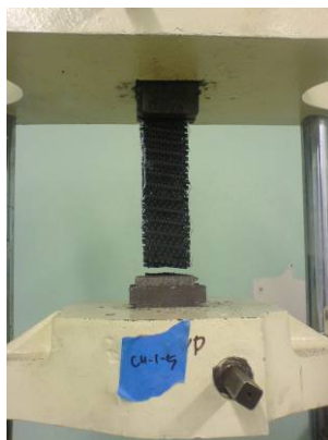
Figure 5.7 Failure Mode of CH-I-5: LWB
