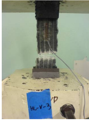
Figure 5.63 Failure Mode of HL-V-3: LWB
