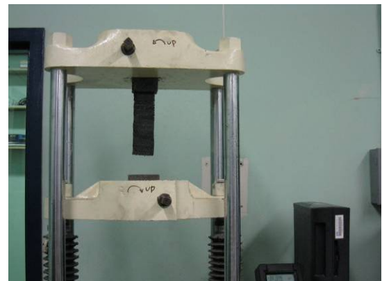
Figure 5.8 Failure Mode of CH-II-2: LWB
