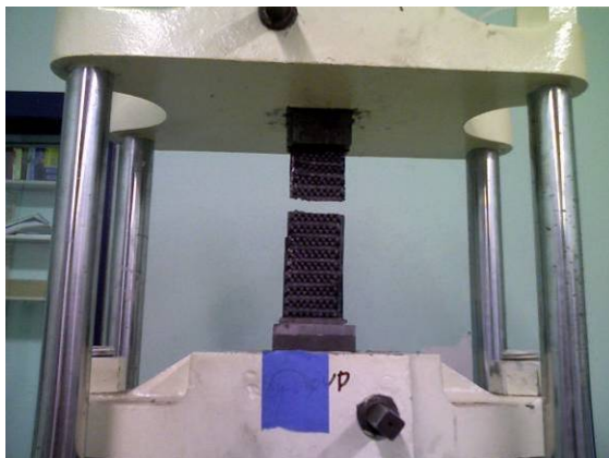
Figure 5.13 Failure Mode of CH-II-7: LGM
