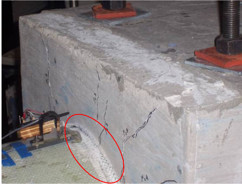
Figure 3.40 Tube Embedment Intact for Specimen G until \mu=3
