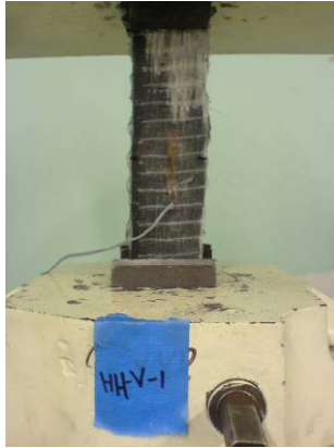
Figure 5.57 Failure Mode of HH-V-1: LAT
