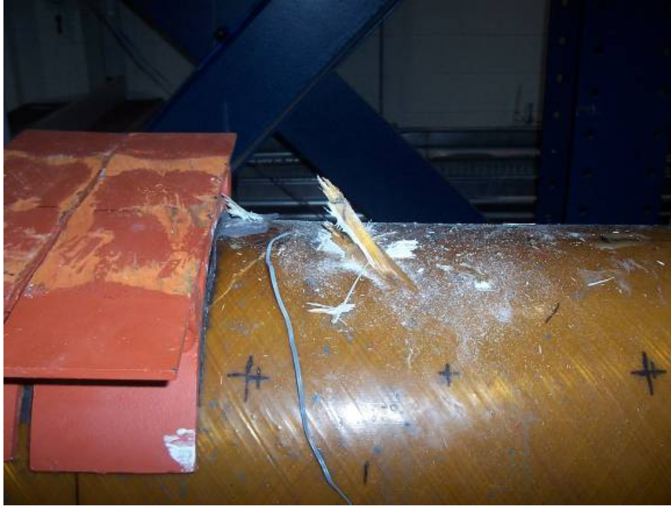
Figure 4.15 Crushing of Specimen Y at the Top (West View)
