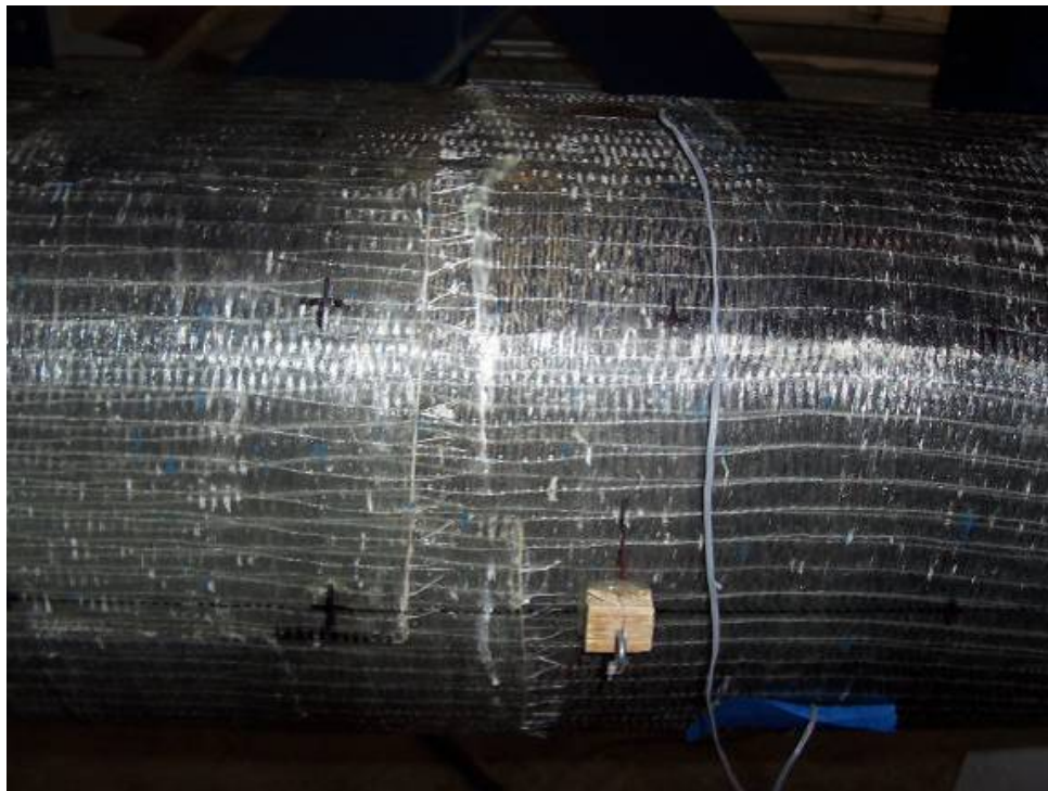
Figure 4.22 Crumpling Crack in Specimen H at the Top (West View)
