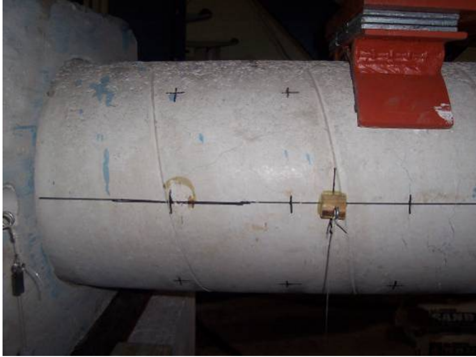
Figure 4.11 Shear Cracks of Specimen RC in Shear-Flexural Region Close to Column Head
