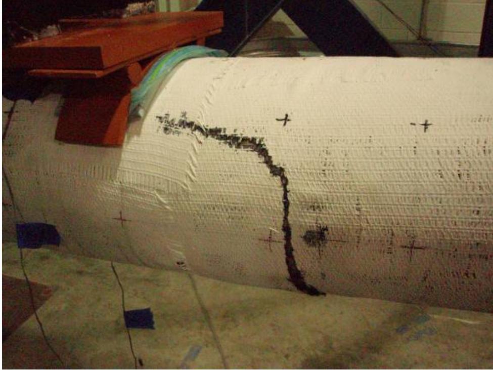
Figure 4.27 Flexural Crack Extended to Mid-Span in Specimen LC (West View)
