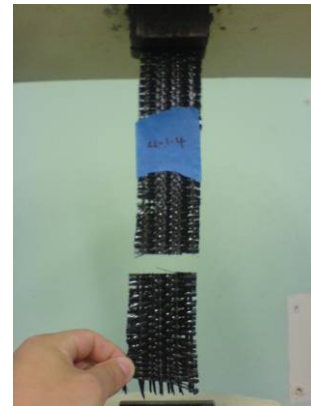
Figure 5.18 Failure Mode of CL-I-4: LIB
