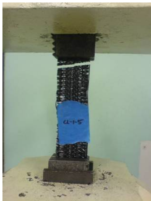
Figure 5.19 Failure Mode of CL-I-5: LWT
