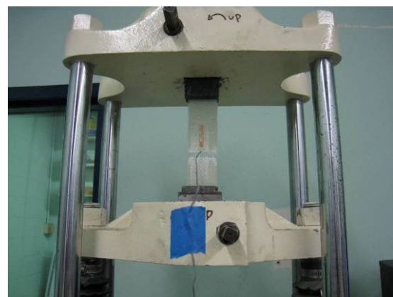
Figure 5.26 Failure Mode of GH-I-2: LGM
