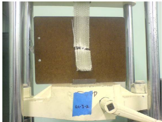
Figure 5.37 Failure Mode of GL-I-2': LAB
