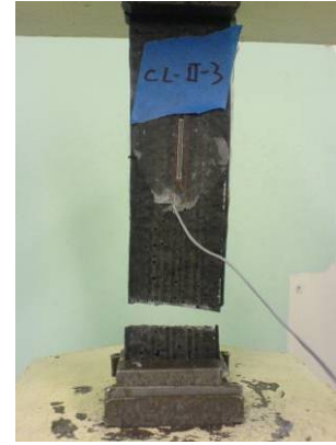
Figure 5.22 Failure Mode of CL-II-3: LAB
