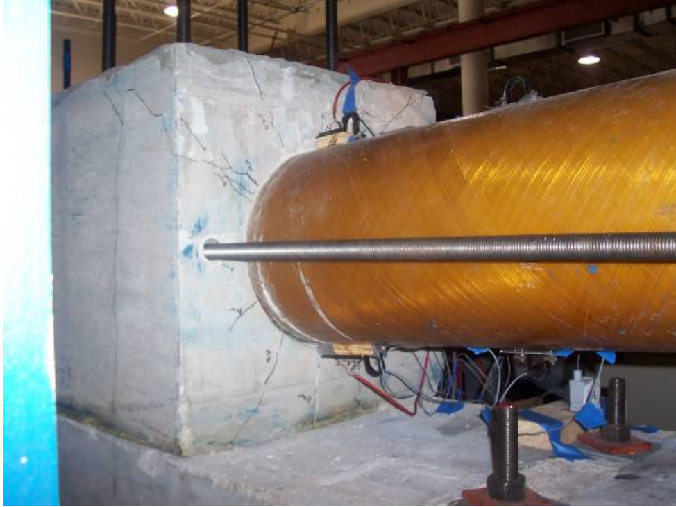
Figure 3.34 Footing Cracks in Specimen Y
