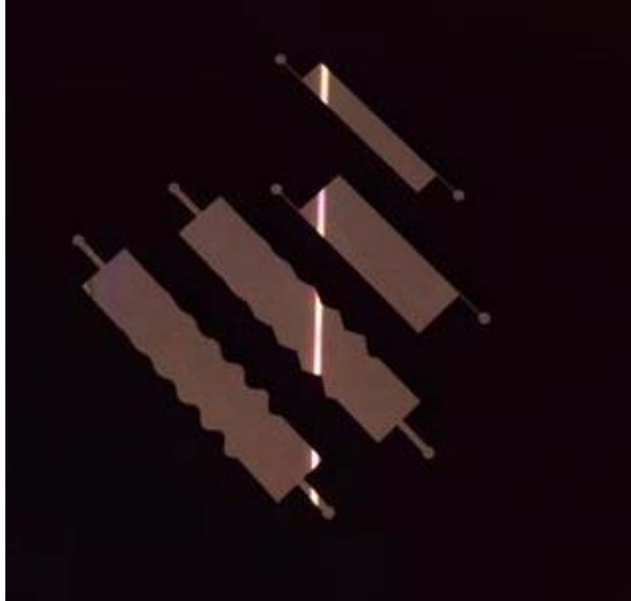
Figure 2.8. Photomask after patterning and before chrome etching.
