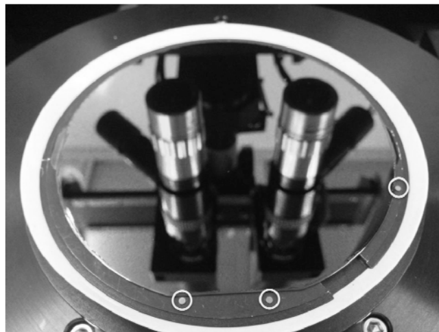
Figure 2.12. Wafer alignment using three pins (inside of yellow circles) on the mask aligner.
