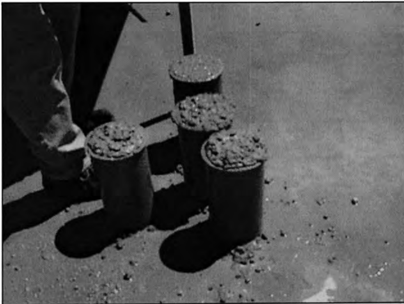
Figure 3.2 Concrete Cylinder Samples
