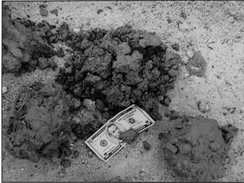
Figure 4.17 Cement Lump Composition
