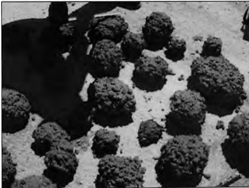
Figure 4.6 Cement Lumps from 7 cuyd Load
