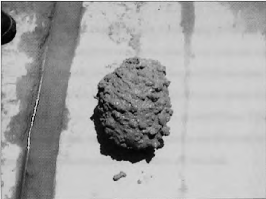
Figure 1.2 Cement Lump or Ball
