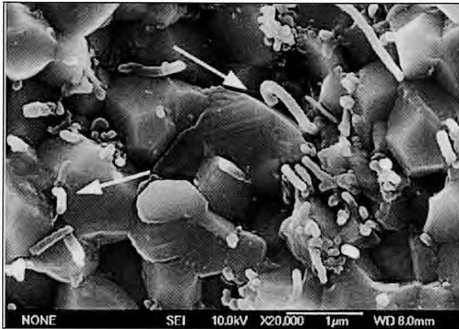
Fig. 2.22: SEM of the fractured surface of Al 2 O 3 -CNT composite sintered at 1450°C showing CNT pullout [11].
