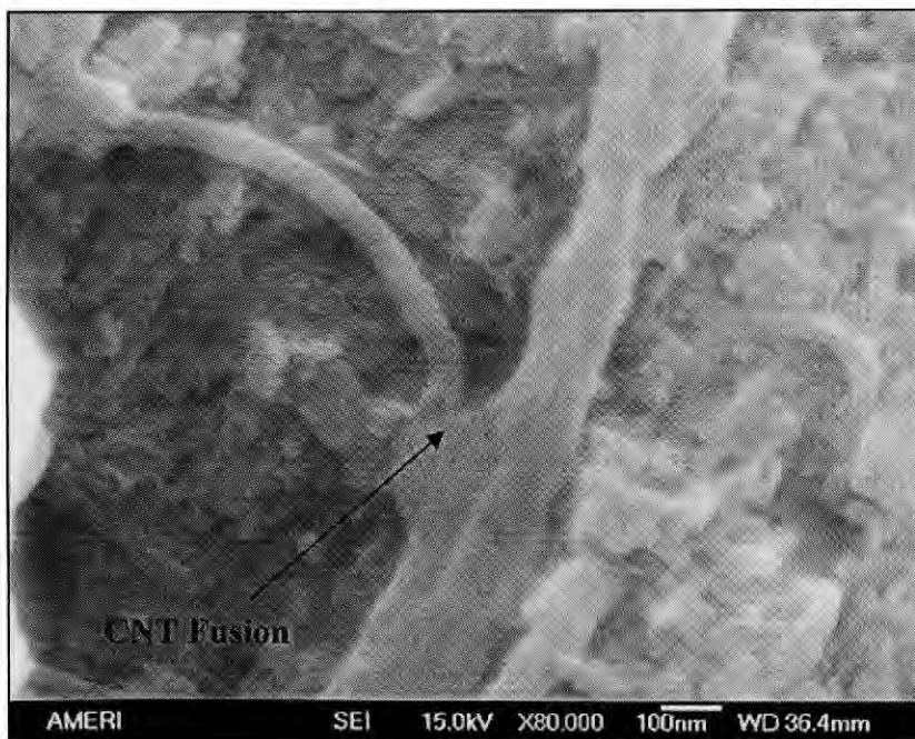
Fig. 4.51: CNT fusion occurring in A8C-SD coating to result a rope structure.
