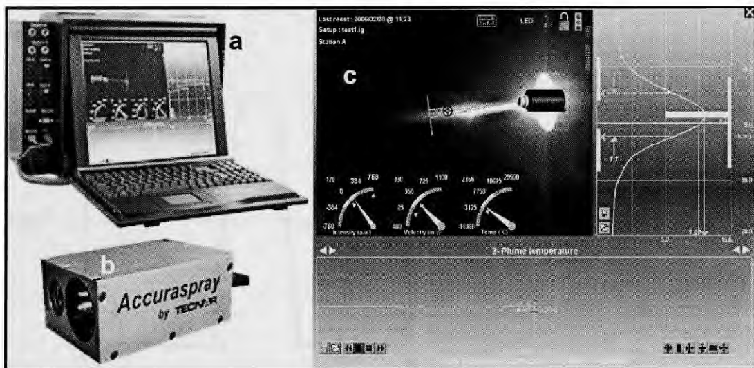
Fig. 3.10: AccuraSpray: Inflight particle diagnostic sensor: (a) Controller with display monitor, (b) the sensor head, and (c) a screenshot showing temperature, velocity and plume profile.
