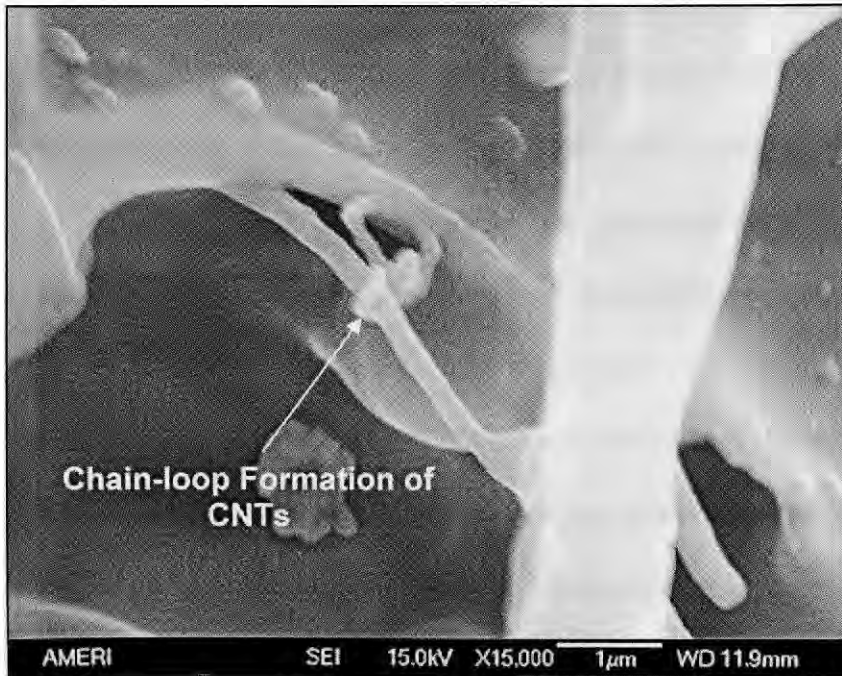
Fig. 4.32: Hook and loop formation of CNTs.
