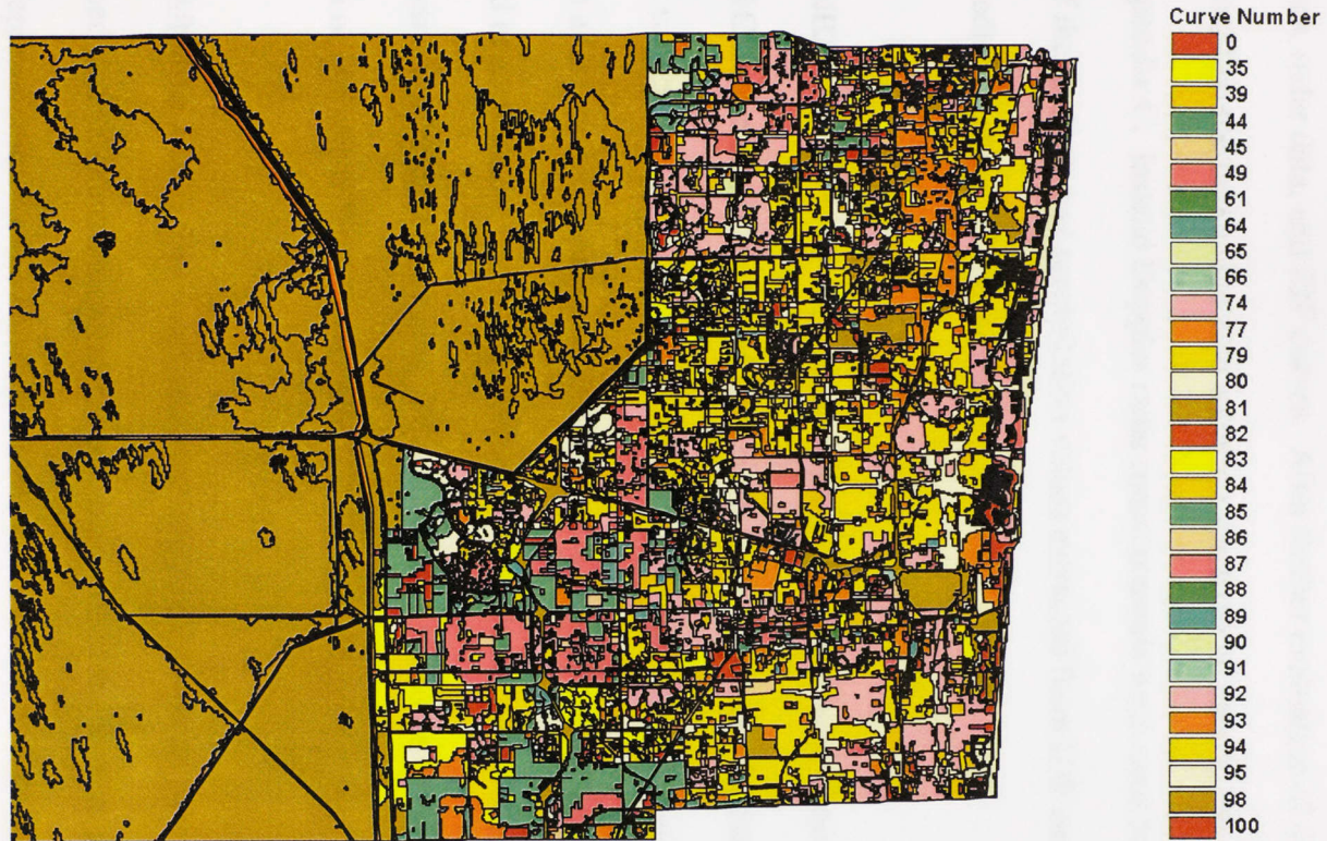
Figure 10. Curve Number values for Antecedent Moisture Condition II, the average soil moisture conditions in Broward County, Florida.
