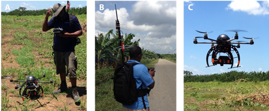
Figure 3.2. Rotary Wing UAV showing (a) approximate size and RC controller, (b) backpack antenna system for location tracking and flight control, and (c) UAV during launch.
