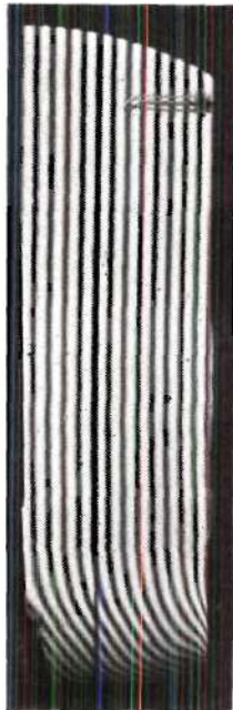
Figure 11. Parallel Fringe Pattern for Simultaneous Heat and Mass Transfer at T_s = 312.6^0\text{K} .
