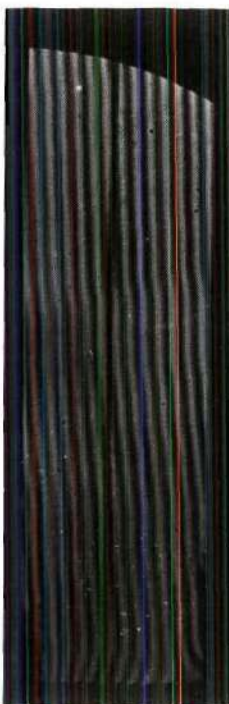
Figure 7. Parallel Fringe Pattern for Isothermal Mass Transfer at T = 303^{\circ}\text{K} .
