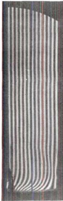
Figure 9. Parallel Fringe Pattern for Heat Transfer Without Evaporation at T_s = 316.5^\circ\text{K} .
