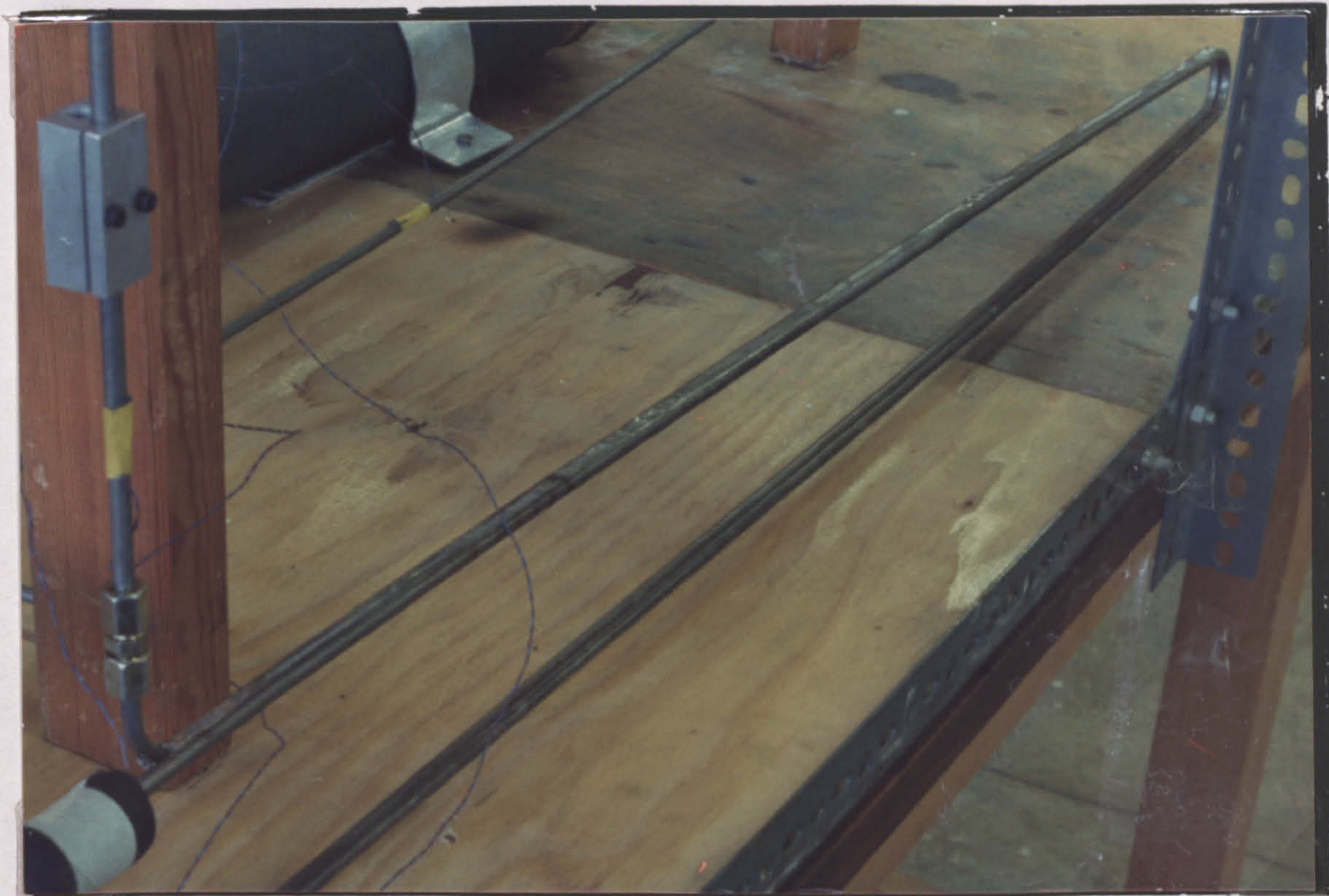
Fig 5.2 Initial experimental apparatus. Top: Apparatus showing separator end on at mid height at left, and receiver end on at a higher level on the right. The tube rising above the separator is the rectifier. The long horizontal cylinder at base level at the back is the reservoir. Bottom: The solution heat exchanger without insulation. At the top left, the resistance heating element acting as a boiler heat source.
