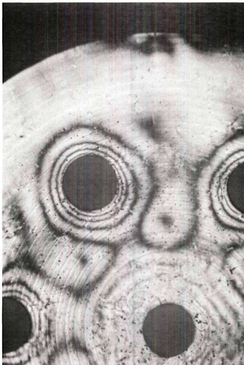
Figure 7. Frozen Stress Pattern for Disk with 9/16 Inch Eccentric Holes (rpm 1680)
