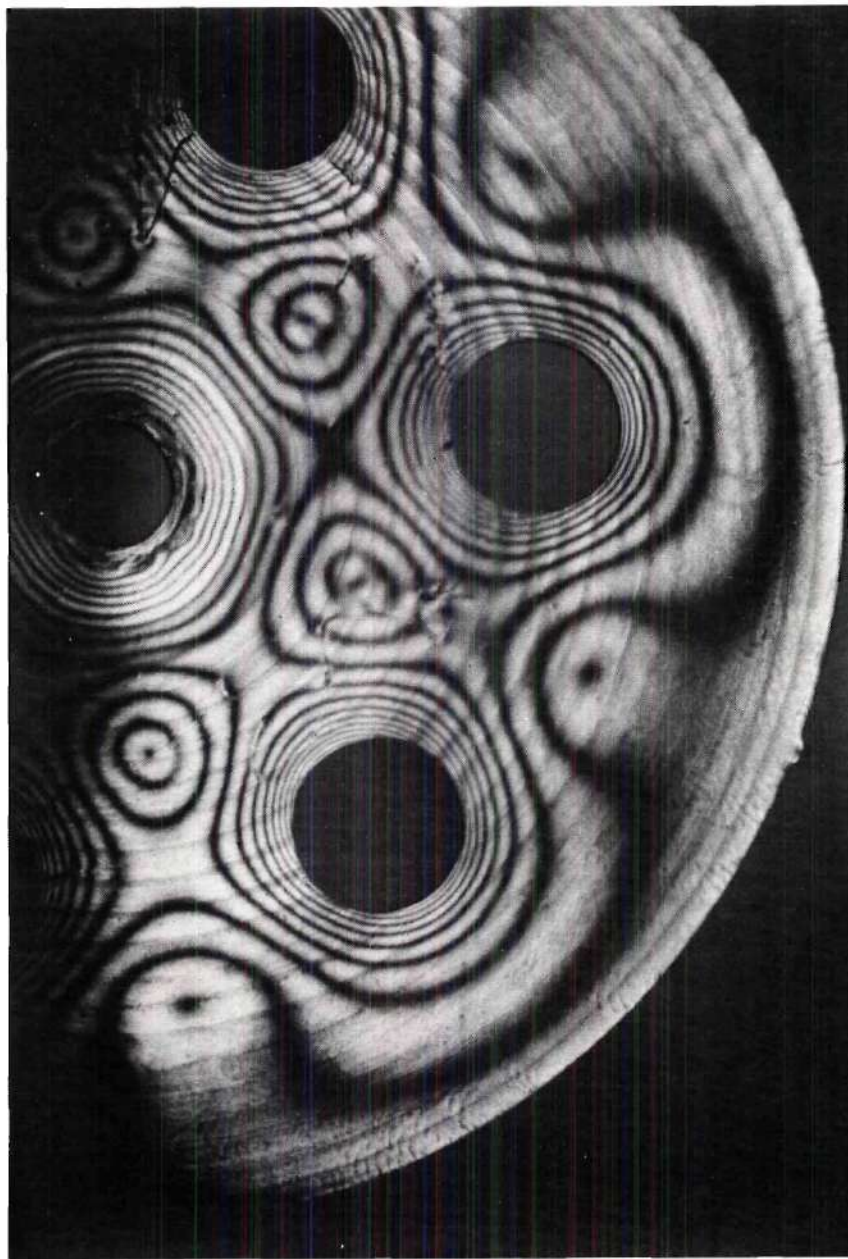
Figure 8. Frozen Stress Pattern for Disk with 3/4 Inch Eccentric Holes (rpm 2670)
