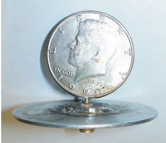
Figure 37: A photograph of the planar disk monopole antenna used for omnidirectional measurements.
