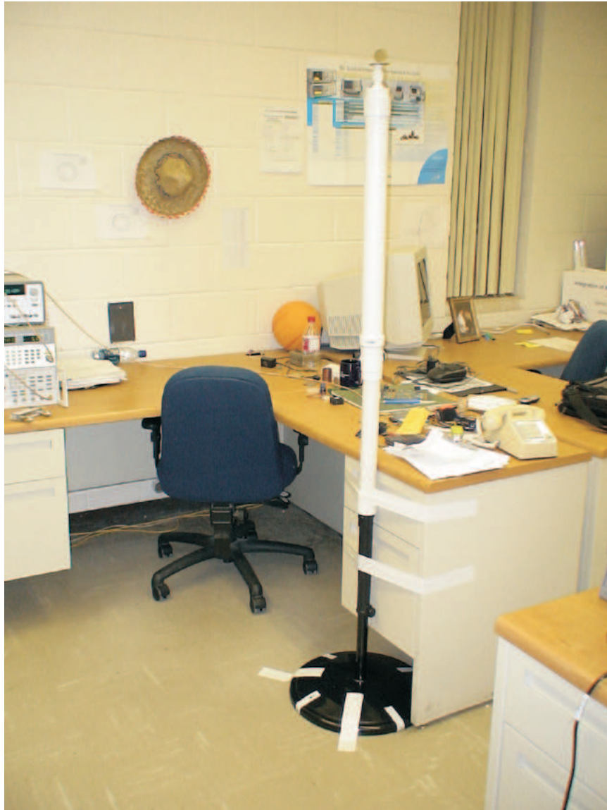
Figure 46: The transmitter was located in a typical office environment with the antenna mounted atop a 180 cm pole.
