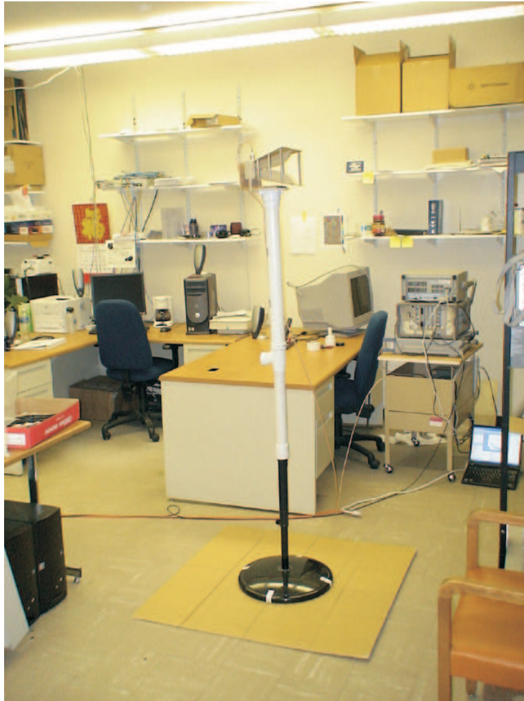
Figure 60: Site C was a LOS measurement approximately 4.8 meters from the transmitter.
