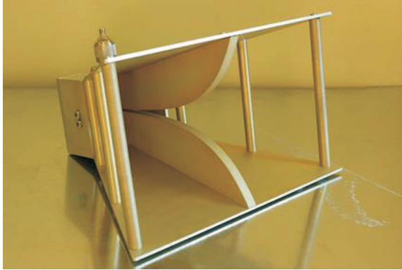
Figure 39: A photograph of the double-ridged horn antenna used for directional measurements.
