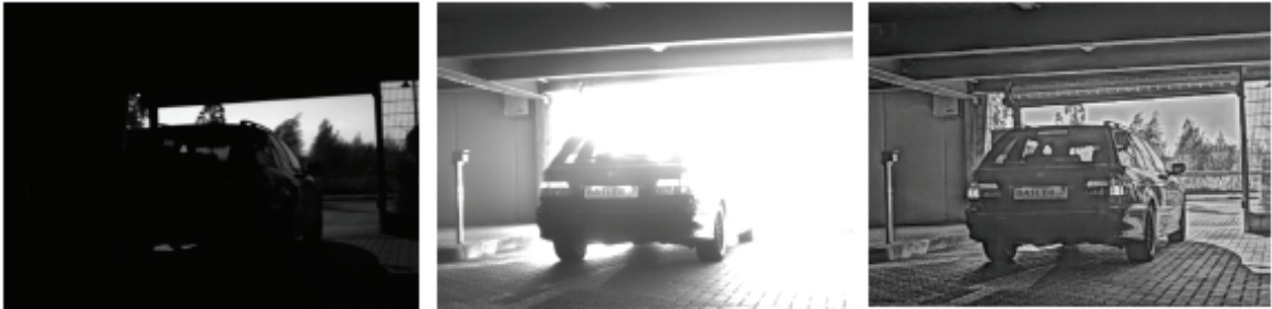
Figure 36: Left: Conventional underexposed image; Middle: Conventional overexposed image; Right: 22-bit high dynamic range camera image [139].
