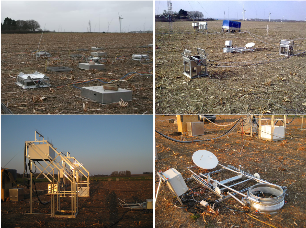
Figure 10.1: Pictures of the \text{N}_2\text{O} flux chamber intercomparison campaign at fieldsite RISØ. Upper left: automated KIT flux chambers (transparent chamber) and manual RISØ chambers (opaque chambers); upper right: automated flux chambers from the University of Bremen; in background the EC tower; lower left: automated flux chambers from Thünen Institute; lower right: automated photosynthesis-flux chambers from RISØ.
