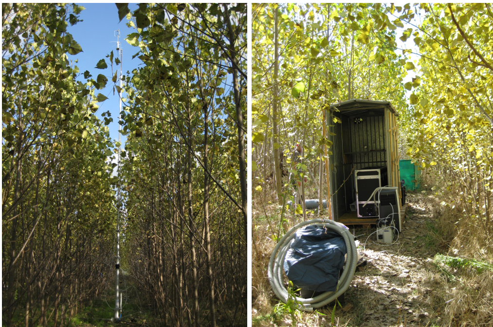
Figure 4.8: Pictures of the set-up at the fieldsite Poplar. Left figure: the tower with the vertical inlets was positioned between two poplar tree lanes. Right figure: the metal housing of the FTIR-analyzer was placed between two poplar tree lanes.
