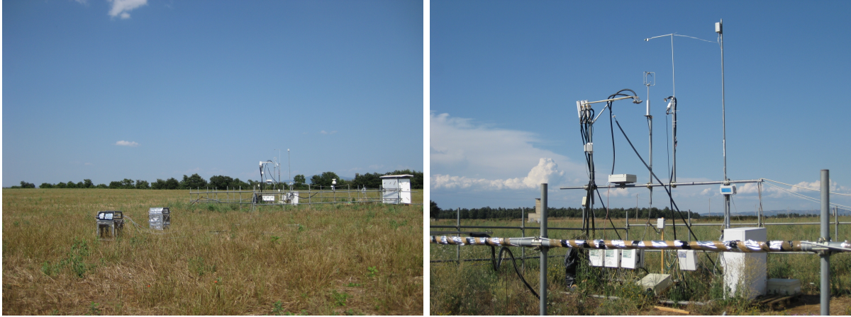
Figure 4.3: Pictures of the fieldsite Rocca4. Left figure: an overview of the fieldsite Rocca4, with in the front the two flux chambers, and in the back the EC tower and the metal housing. Right figure: the EC tower with the FG inlets and the small pumps at 1.30 and 4.10 m. The fence is against cattle, which usually graze in this fieldsite.
