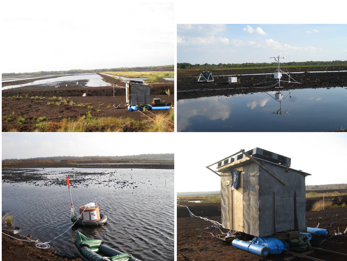
Figure 4.2: Pictures of the measurement set-up at the fieldsite Himmelmoor. Upper left: the view of the set-up in the rewetted area (light green zone, Figure 4.1); upper right: the FG tower in the rewetted area; at the end of the experiment, the FG tower was inside a water pond. Lower left: picture of the floating chamber experiment (see §10.3.1), lower right: the wagon wherein the FTIR-analyzer, the UPS and sampling box were placed.
