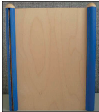
Figure 5.3: One of the two objects that have a notch on both sides. Other objects can be slid into these notches in order to be fastened.
