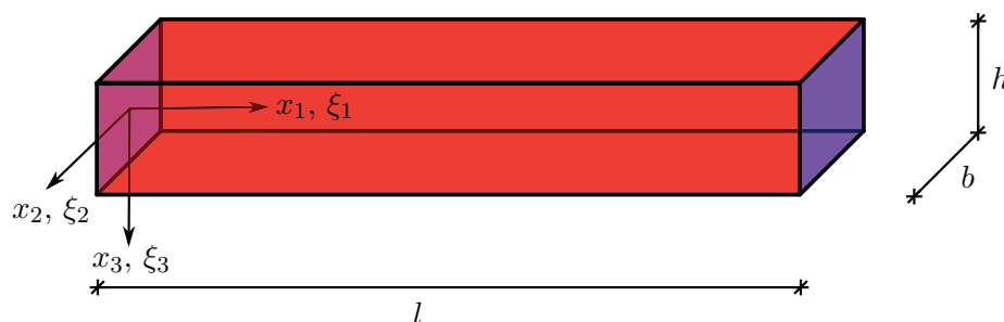
Figure 2: The beam geometry. On the (blue) face sides either displacement boundary conditions or traction boundary conditions are prescribed. On the (red) lateral sides traction boundary conditions are prescribed. The directions of the boundary tractions g , the volume force field f and the prescribed displacements u_0 are not restricted.
