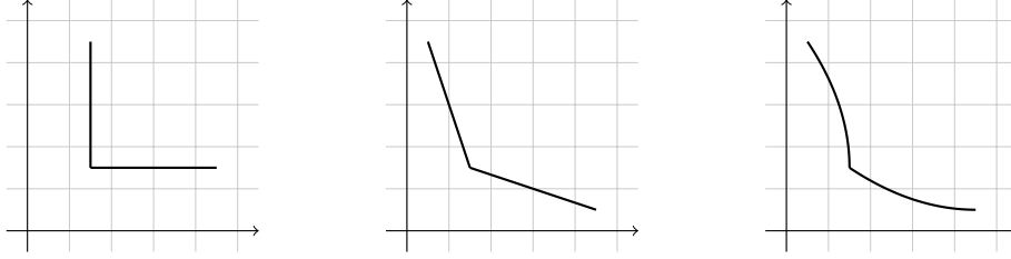
Figure 5.2: Perfect L-curve of order N for N = 0 (left), N = 1 (center) and N = 2 (right).
