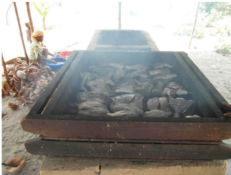
Figure 2.8 Improved technology of fish smoking to reduce fuel wood consumption in Msimbati village
