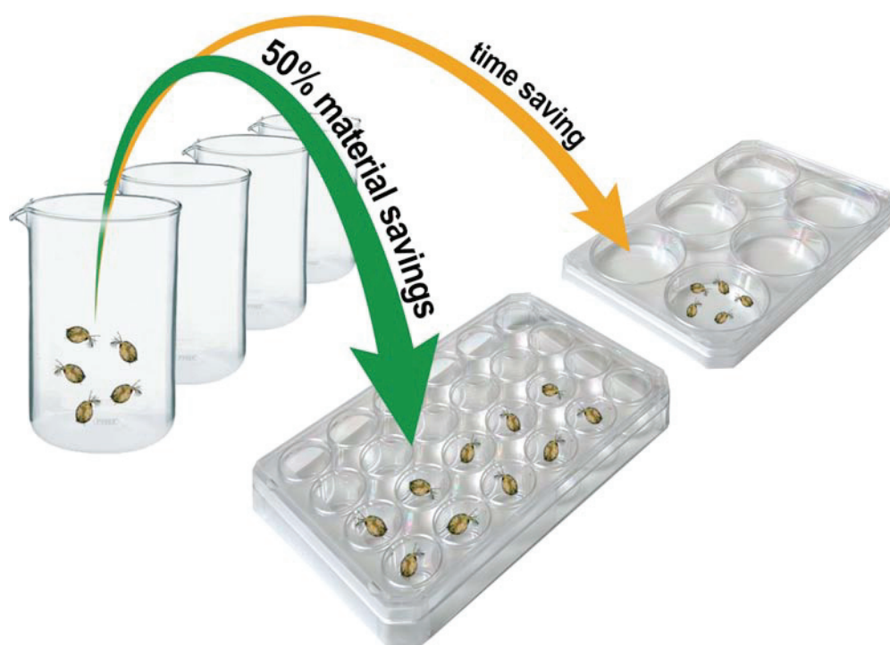
Fig. 5: Scheme of the miniaturization of the Daphnia sp. acute toxicity test presented in publication 1. Due to the performance in 24-well microtiter plates, 50 % of animals and test substances can be saved compared to the OECD standard test. Alternatively, the performance of the standard test was tested in 6-well microtiter plates, which still allows remarkable time savings.
