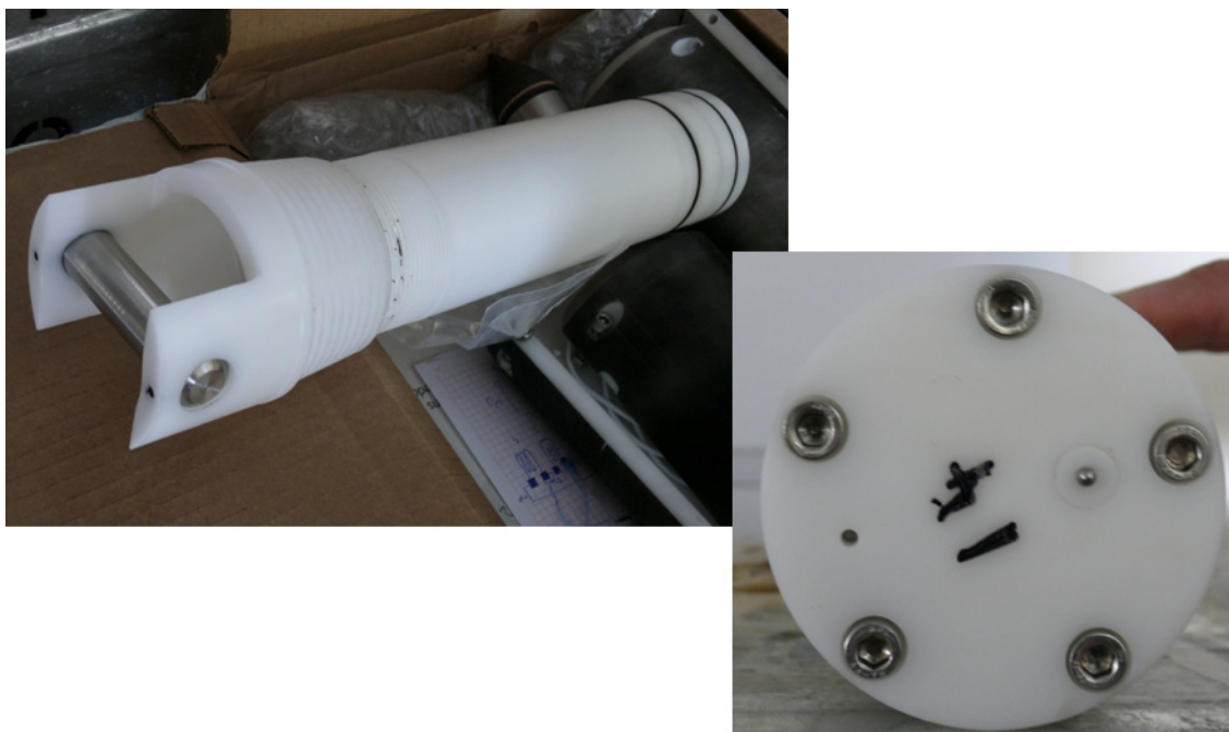
Figure 5.25: Left: MeBoPlug prior to being screwed into a MeBo drill pipe Right: bottom view into the borehole with ports for P [hole at left] and T [little pin at right] monitoring. See text.
