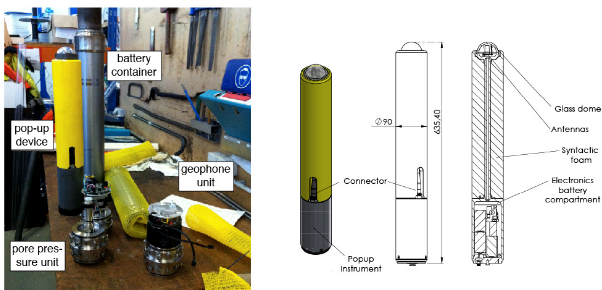
Figure S.30: Schematic diagram ( left ) and photograph ( right ) of MeBoPUPPI observatory
