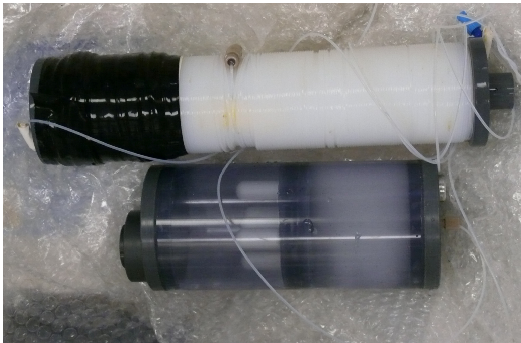
Figure S.29: OsmoSampler (tubing coil [top] and pumps [below]) that are hosted in a PVC tube attached to MeBoCORK-B.
