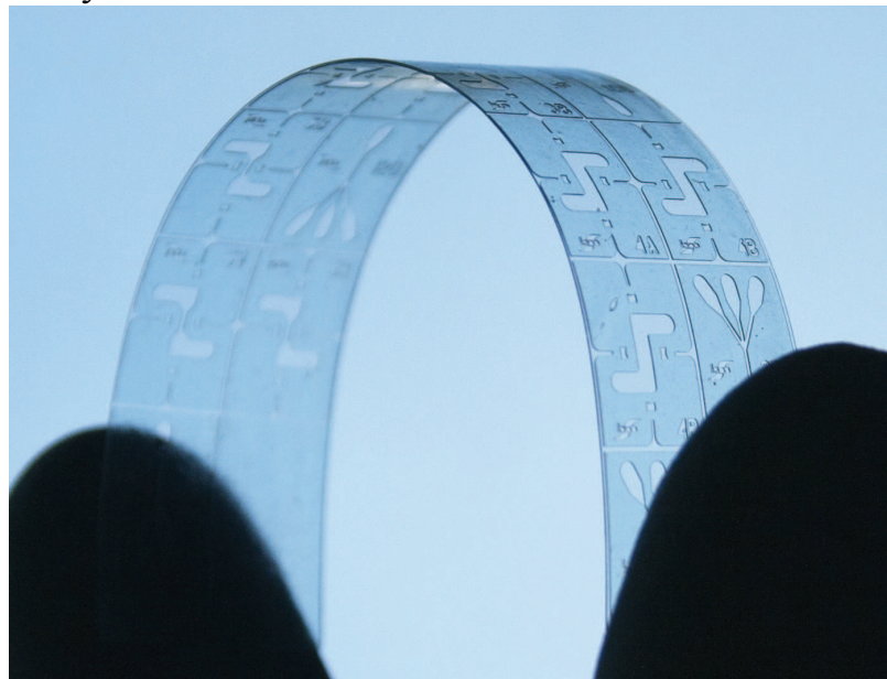
Figure 3.10: Photograph of fabricated devices before cutting and bonding. The microfluidic and optical elements are structured in dry resist. A polyester foil is used as substrate.
