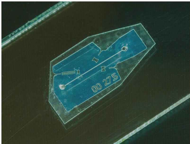
Figure 6.9: Photograph of the device for the analysis of liquid concentrations. A dry film resist is structured on a polyester foil and bonded to PMMA microscope slide.
