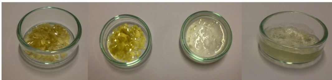
Abbildung 3.11: links: ungequollenes Polymer, rechts: in Aceton gequollenes Polymer
