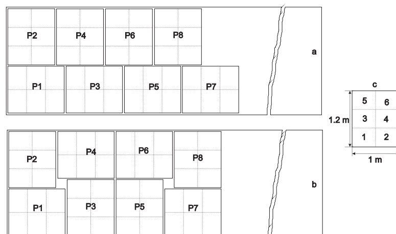
Figure 5.7: (a) The standard scheme layout of pallets in the container, (b) the chimney layout of pallets in the container and (c) top view of a pallet shows the six boxes on the top layer.
