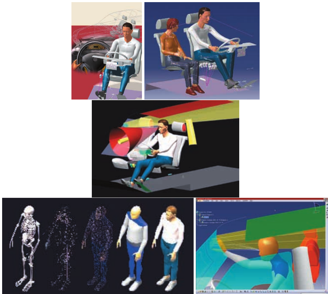
Figure 2.6: RAMSIS 3D-CAD-ergonomics tool presenting geometric kinematic digital human model (Source: Human Solutions GmbH [2012] )
