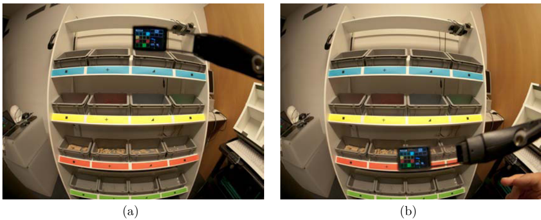
Figure 39: The MicroOptical SV-6 can be positioned outside of the normal line of sight. Note that the field of view of the camera lens is nearly 180^\circ (in the diagonal), which is higher than the field of vision of a human.
