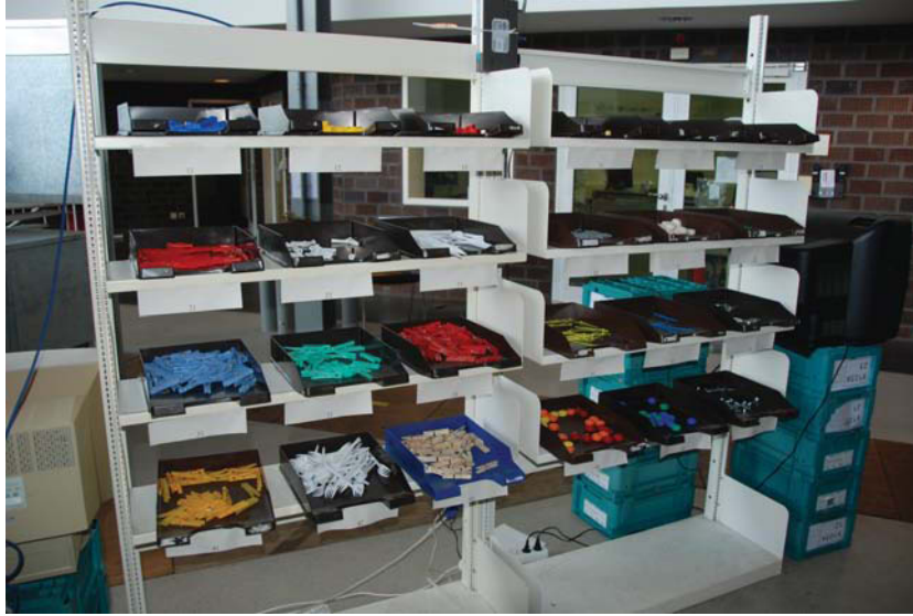
Figure 4: Arrangement of parts and shelves. Two sets of shelves, A and B, each contains 4 rows of 3 part bins.
