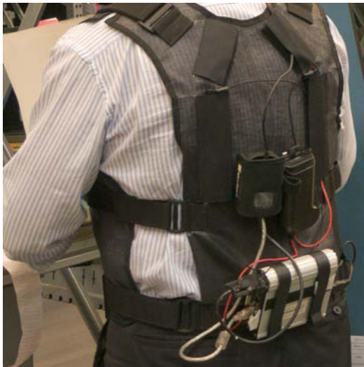
(a) Back: wearable computer, HMD electronic, battery, wlan-antennas
