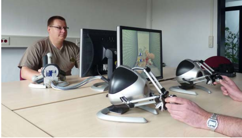
Figure 7.17: The two-player set up with four haptic devices for our user study
