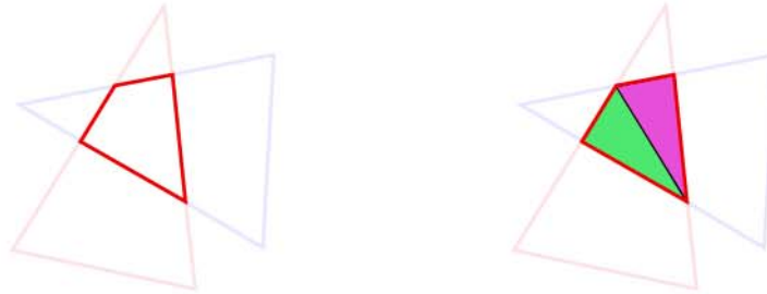
Figure 5.18: Our tetrahedron intersection method: the second step we tetrahedralize the resulting polyhedron.
