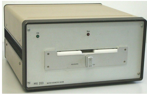
Figure 3.1: Wafer geometry gauge Eichhorn & Hausmann MX-203 [66]
