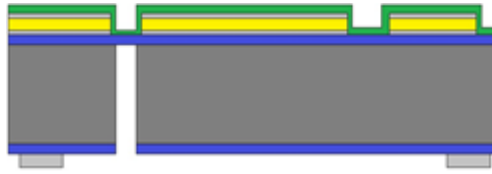
Figure 3.24: Microvalve flow: PECVD of Si 3 N 4 isolation
