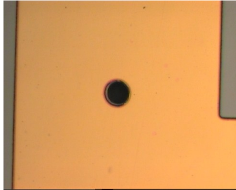
Figure 3.25: Gas inlet from the top side
