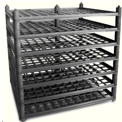
Abb. 5: Chargiergestell aus CFC-Material [Gra2011]
