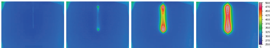
Figure 6.18: From left to right four pictures of the temperature distribution in agar gel during the ablation are depicted. On the right a scale for the temperature in ^{\circ}\text{C} is shown.
