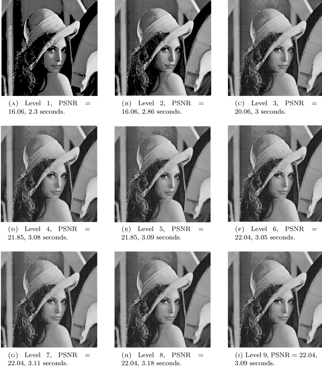
FIGURE E.2.1. Reconstructed image for wavelet based on the Sierpinski Gasket for different levels.
