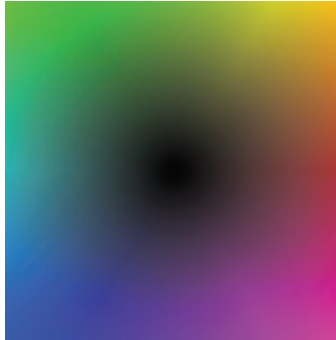
Figure 1.1: Color coding map of the optical flow: Direction is coded by hue, length is coded by saturation.
