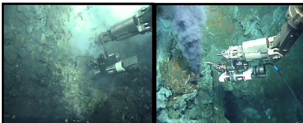
Figure 7.1 Typical deployment of the IGT samplers with the starboard ROV manipulator: (left) sampling of a 104°C white smoker fluid at North Su during Dive 316 (S051) and (right) sampling of a 304°C black smoker (after excavation of the structure shown in Fig. 6.12A) on the flank the Fenway mound (PACMANUS) during Dive 305 (S025).
