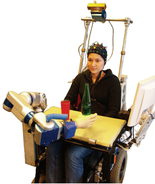
Figure 4.1.: Rehabilitation robot FRIEND-II controlled by the Bremen-BCI.
