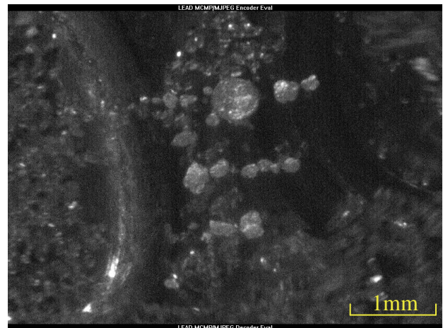
(b) gold trapped in 120 seconds with electric field
