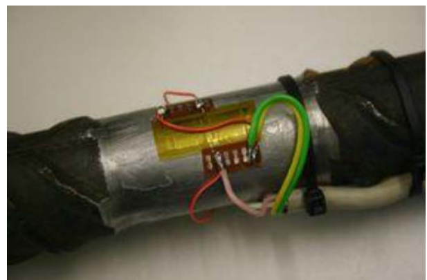
Figure 5. DMS on reinforcement bar [15]
