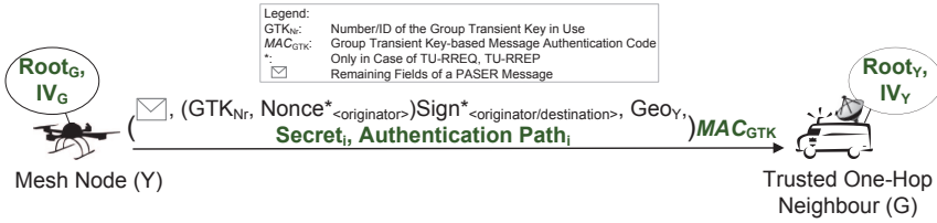
Figure 5.9: Symmetric scheme for secure communication between trusted one-hop neighbors in PASER [Sbe15].
